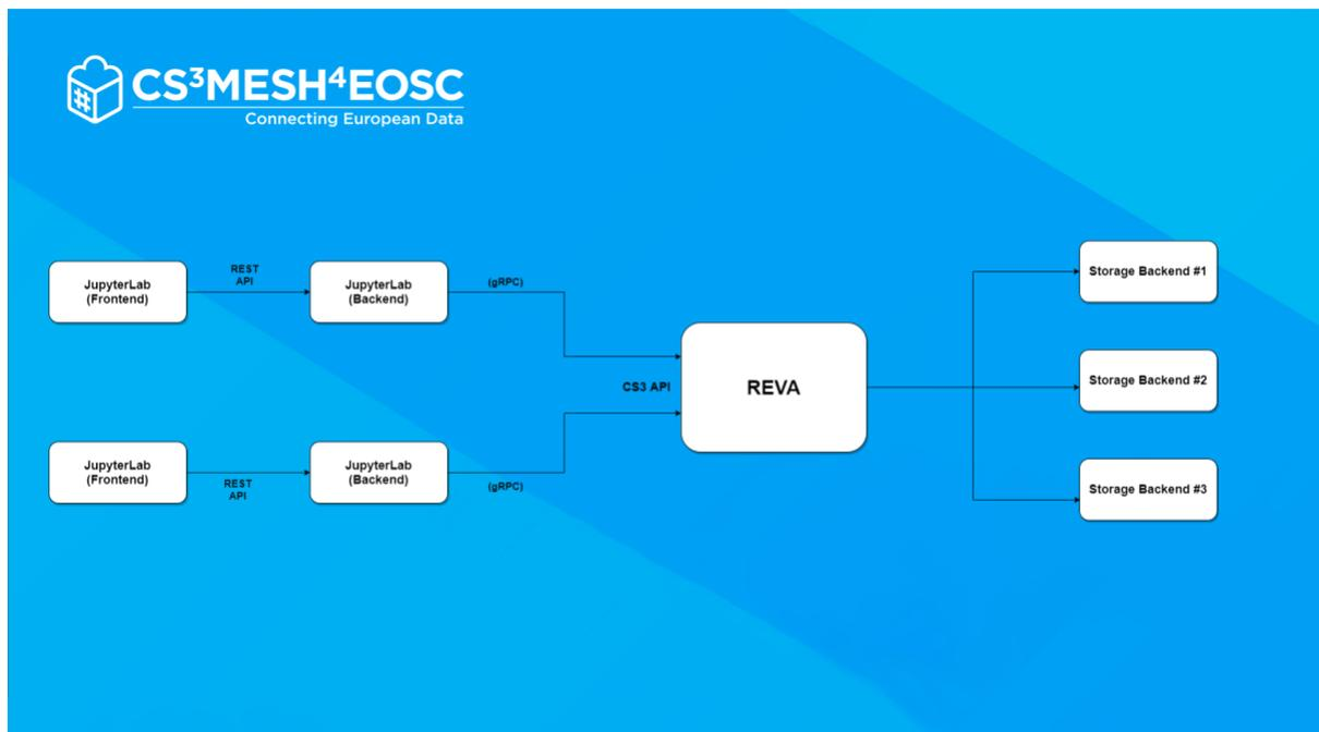
Figure 8. JupyterLab integration with IOP/Reva
