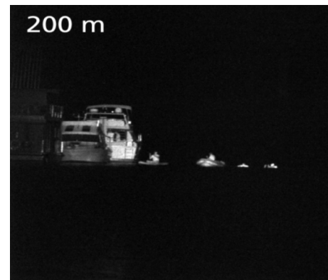
Fig. 6. A captured picture with objects reflecting the illuminated light at a distance of 200 meter.
