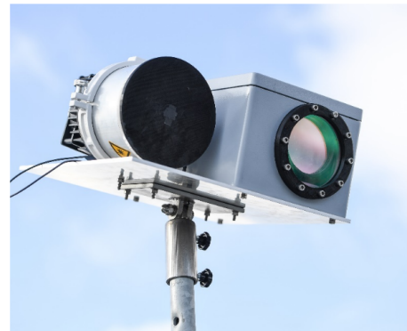
Fig. 5. The TRAGVIS sensor with the illuminator (left) and the synchronized camera (right).
