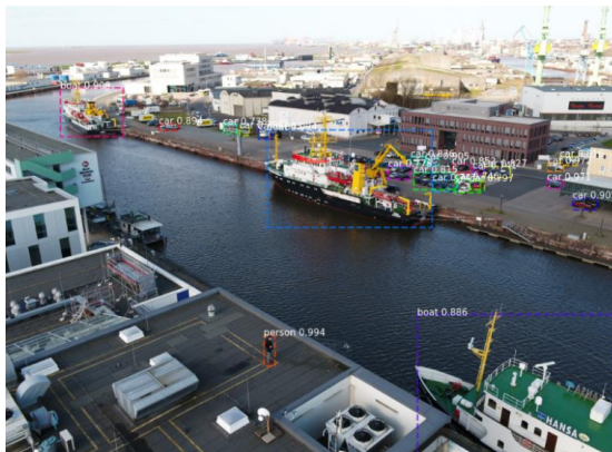
Fig. 4. Example image of detected persons, cars and vessels from a video stream like from the HarbourCam. Geo-referencing the detections allows to draw shapes on a map corresponding to the location (see Fig. 9).
