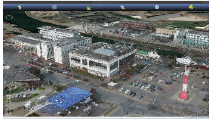
Fig. 8. A pointcloud of our institute's building generated out of the drones imagery. It is shown in the situational awareness software developed in the MARLIN project.
