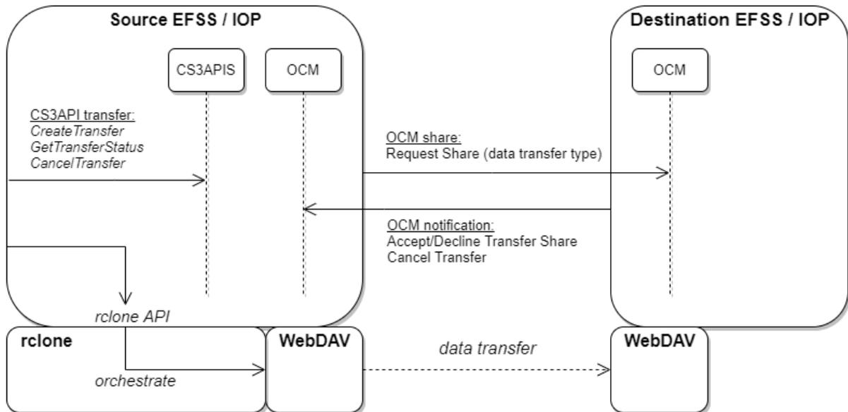
Figure 9. Direct file transfer between source and destination EFSS/IOP is supported through CS3APIS and OCM interfaces, rclone, and WebDAV.
