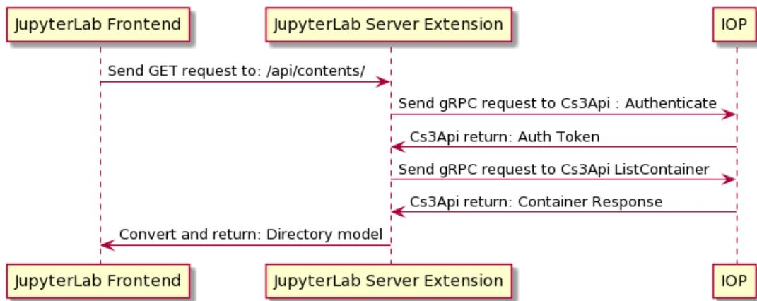
Figure 6. An example of reading a directory from an IOP using the JupyterLab extension
