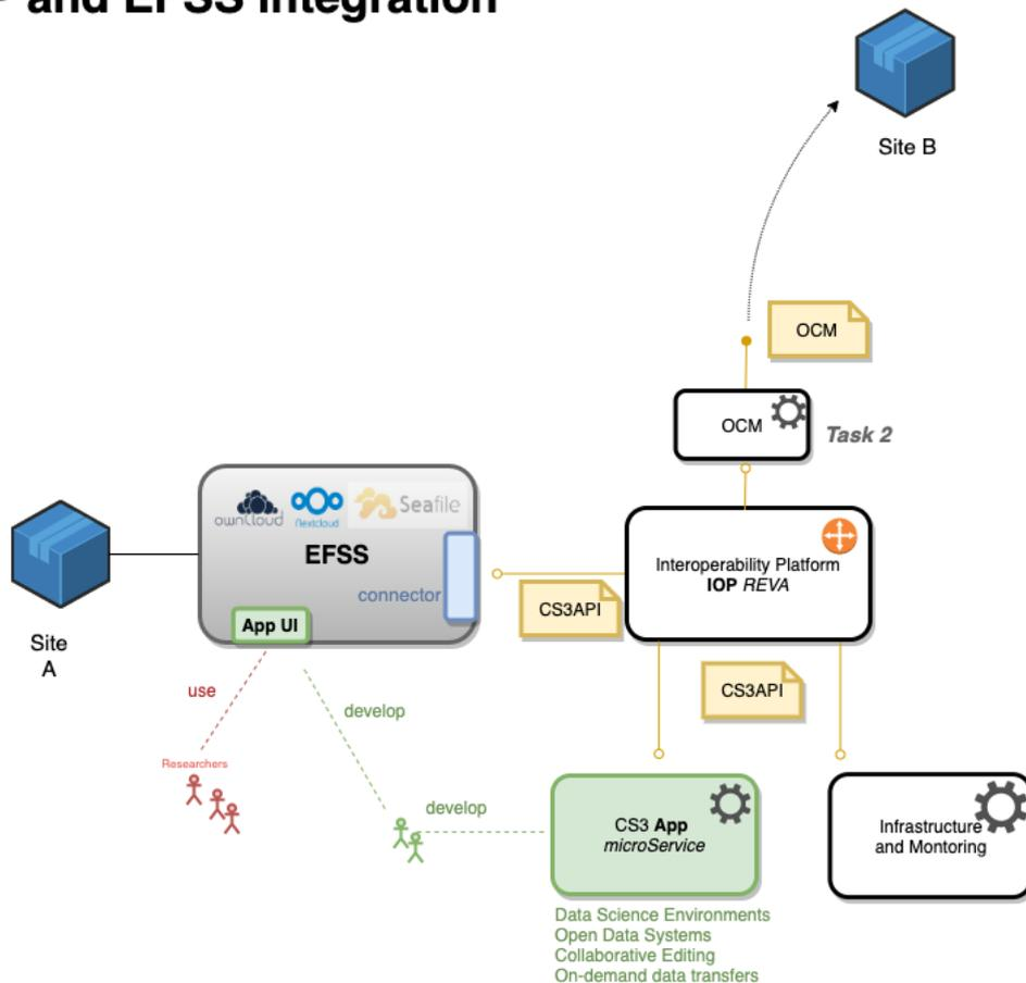
Figure 4. IOP and EFSS Integration Architecture
