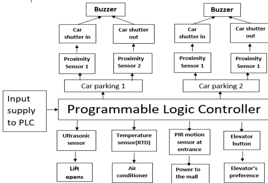
Fig. 1. Block diagram of Hardware Setup for Simulation Working
