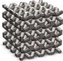
Fig. 1. Schematic of lattice structure cube specimen.
