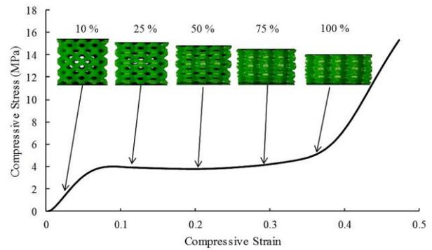
**Fig. 4. Crush behaviour of FDM ABS lattice structure.**
