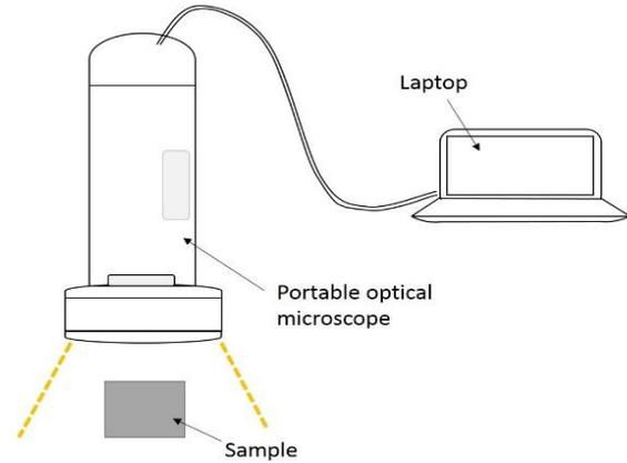
Fig. 2. Portable optical digital microscope.
