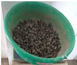
Figure 1. Coarse aggregate
