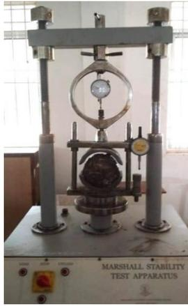
Figure 5, Marshall Stability test on samples
