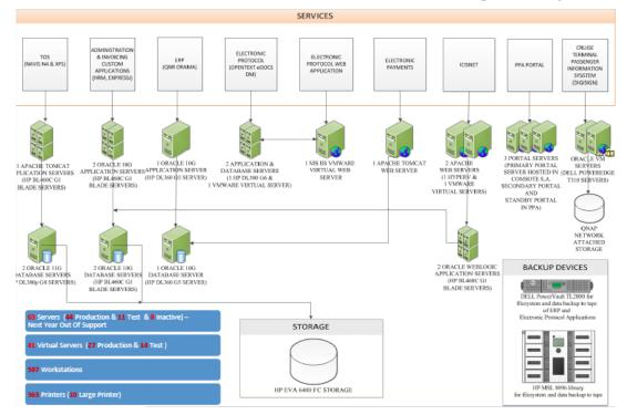
Figure 51. Server and storage structure in Port of Piraeus network
