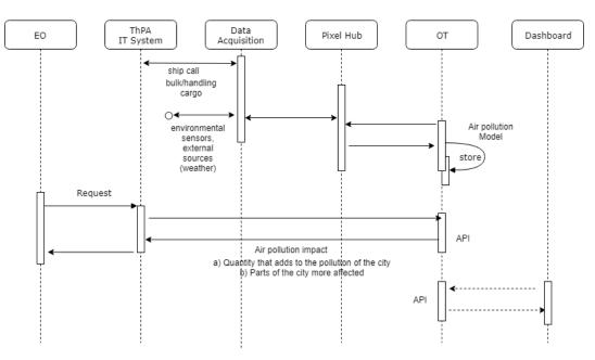
Figure 21. Environmental manager at ThPA. Sequence diagram
