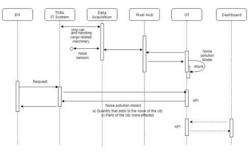
Figure 22. Environmental manager at ThPA (II). Sequence diagram
