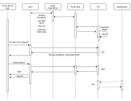
Figure 11. Gate Manager at PoM. Sequence diagram
