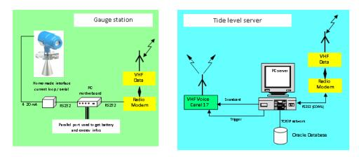
Figure 25. Architecture of gauge station and the tide level server
