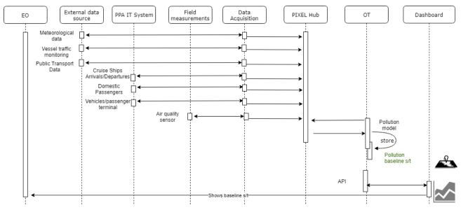
Figure 17. Environmental manager at PPA. Sequence diagram
