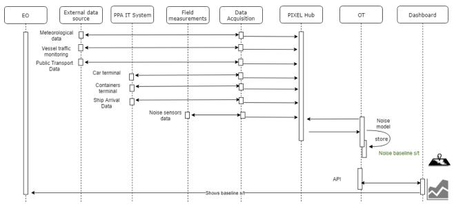
Figure 18. Environmental manager at PPA (II). Sequence diagram
