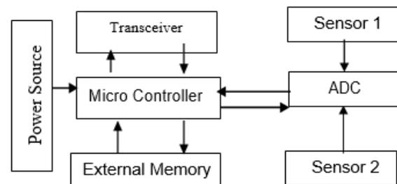
**Figure .2 Sensor node's components**
