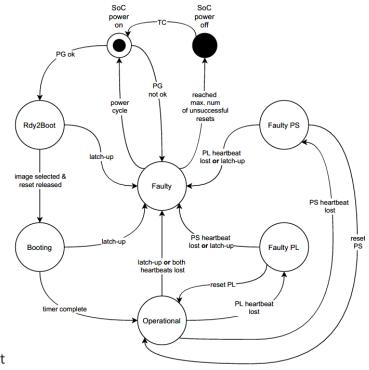
Simplified state machine controlling MPSoC boot and monitoring
