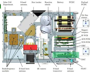
EIVE 6U cubesat (credit: IRS Uni Stuttgart); multiMIND PCB stack in green rectangle, labelled as DAC [mission board] and PLOC
