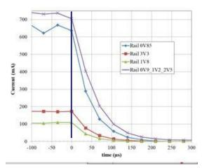
Self-monitored MPSoC power down (data available via TM link afterwards "test-while-you-fly")
