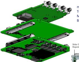
multiMIND PCB stack for EIVE (exploded view): Top: COTS FMC board ("frontend") Mid: mission board, holding FMC I/F and satbus I/F Bot: multiMIND code board; heat dump to the bottom
