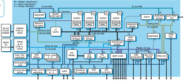
Cobham Gaisler digital IP: LEON4FT and IO peripherals
