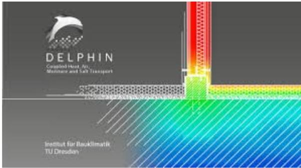
DELPHIN 6.1 is a software tool developed at University of Dresden that allows a detailed 2-D numerical study of the dynamic heat and mass transfer phenomena inside building components, including **vapour diffusion, vapour and liquid sorption and capillary suction**
