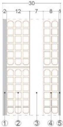
Starting from this wall configuration, **further layers are applied on the outer side** according to the e-CLT solution ( $U = 0.28 \text{ W}\cdot\text{m}^{-2}\cdot\text{K}^{-1}$ ):
