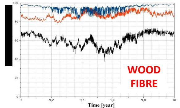
➤ In Milan RH keeps constantly  $\geq 90\%$  both in the CLT and in the wood fibre, while in Catania it ranges between 40% and 70%
