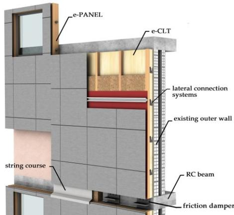
**e-CLT integrates** both **local bio-based recyclable (or recycled) insulating materials** and customizable cladding finishing solutions. Size and number of CLT panels to be applied on the façade are determined based on the initial seismic deficiency of the building and the assumed target performance
