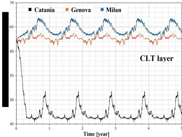
➤ The **TWC in Catania is much lower than in the cold climates** for both layers. Catania is also the only context where the structures dry starting from their initial water content
