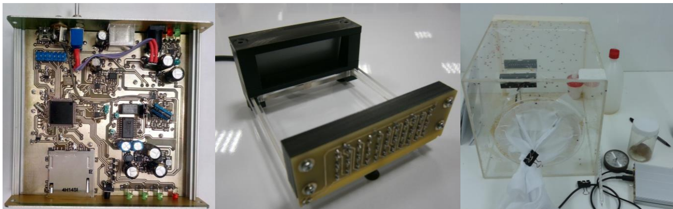
Figure 6. Sensors and system. (Left) The recorder. (Middle) The light-guide aperture inside a dark box providing shade and sitting on 1D array of diodes. (Right) 2D array of diodes sensor and system in their final position in an insectary cage.
