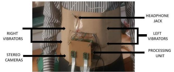
**Figure 2 : Designed mobility aid prototype**
