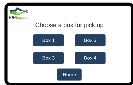
Fig. 6. The baseline Android tablet application for selecting box to be picked up by the robot
