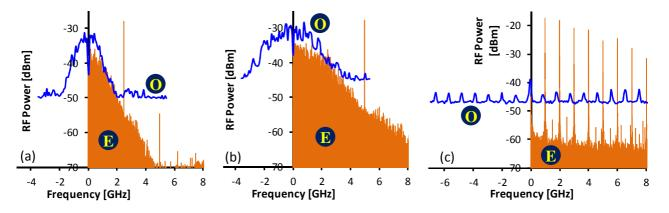
Fig. 4 (a) Acquired signal spectra for (a) 2.5 Gb/s OOK, (b) 5 Gb/s OOK and (c) 1-GHz pulsed clock.
