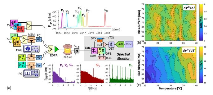
Fig. 2 (a) Experimental setup to evaluate the spectral monitor. The insets show the received optical spectrum and the electrical signal spectra at the particular channels. EML tuning efficiency for (b) current tuning and (c) temperature tuning.
