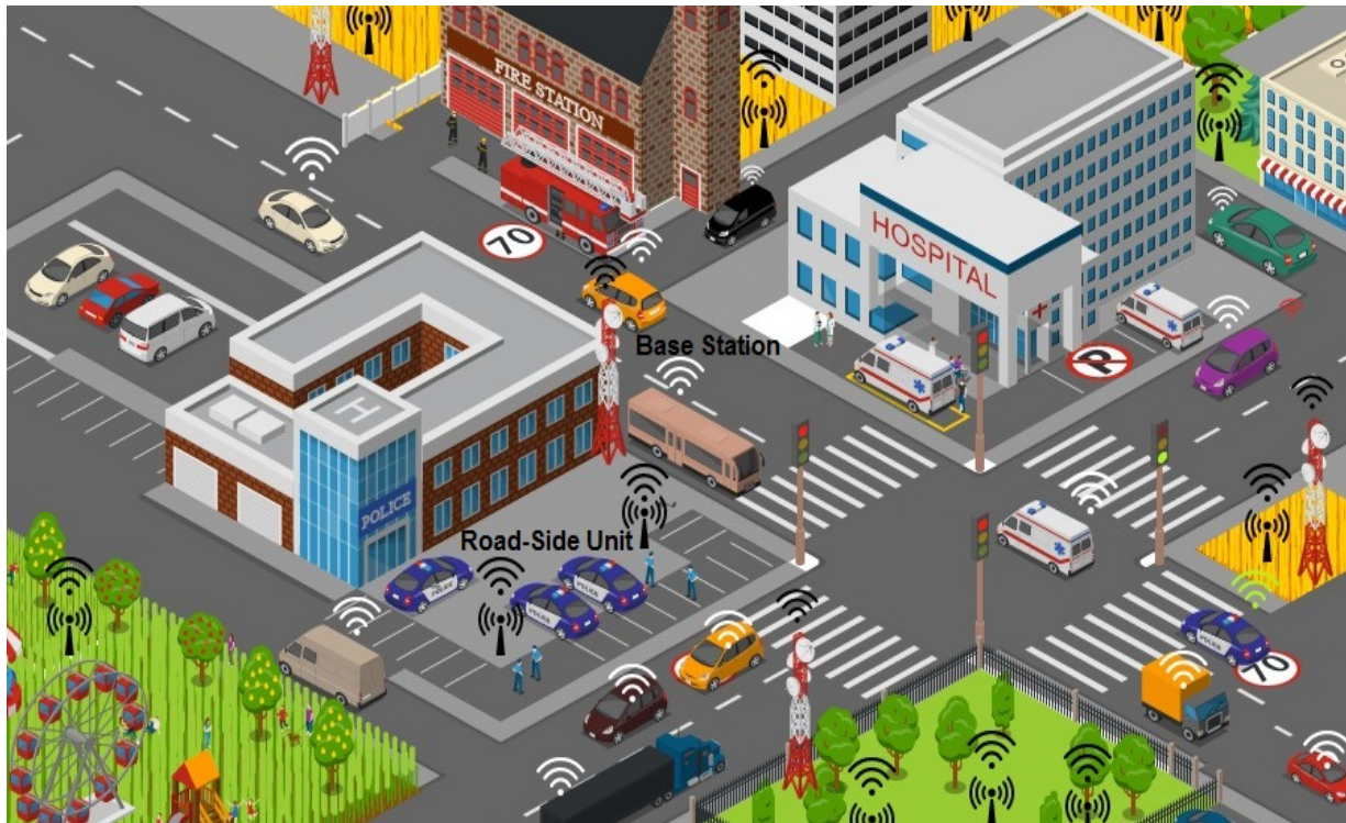
Figure 3. VANET Transmission using DSRC.
