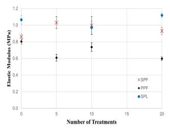
Fig. 7. Effect of the number of soap and water treatments on latex gloves' elastic modulus.
