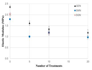
Fig. 5. Effect of the number of soap and water treatments on nitrile gloves' elastic modulus.
