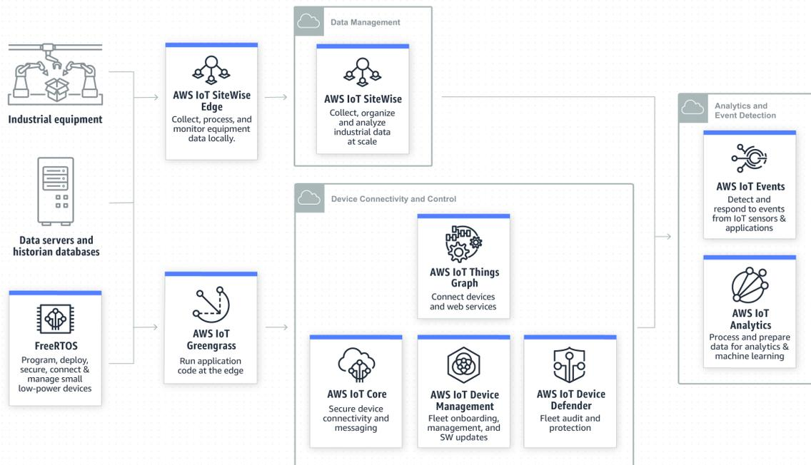
FIGURE 22: AWS IoT ARCHITECTURE – SOURCE: AMAZON.
