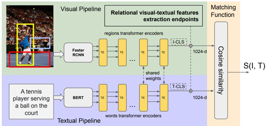
**Fig. 2.** Overview of the TERN architecture. Orange boxes are Transformer Encoder (TE) layers. Final TE layers share their weights for better stability during the training phase. (Color figure online)
