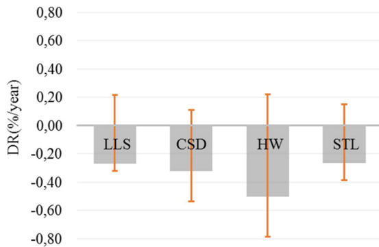
Fig. 13. Annual degradation rate and the uncertainty by applying linear fitting on PR time series (LLS) and trends from CSD, HW, and STL method.
