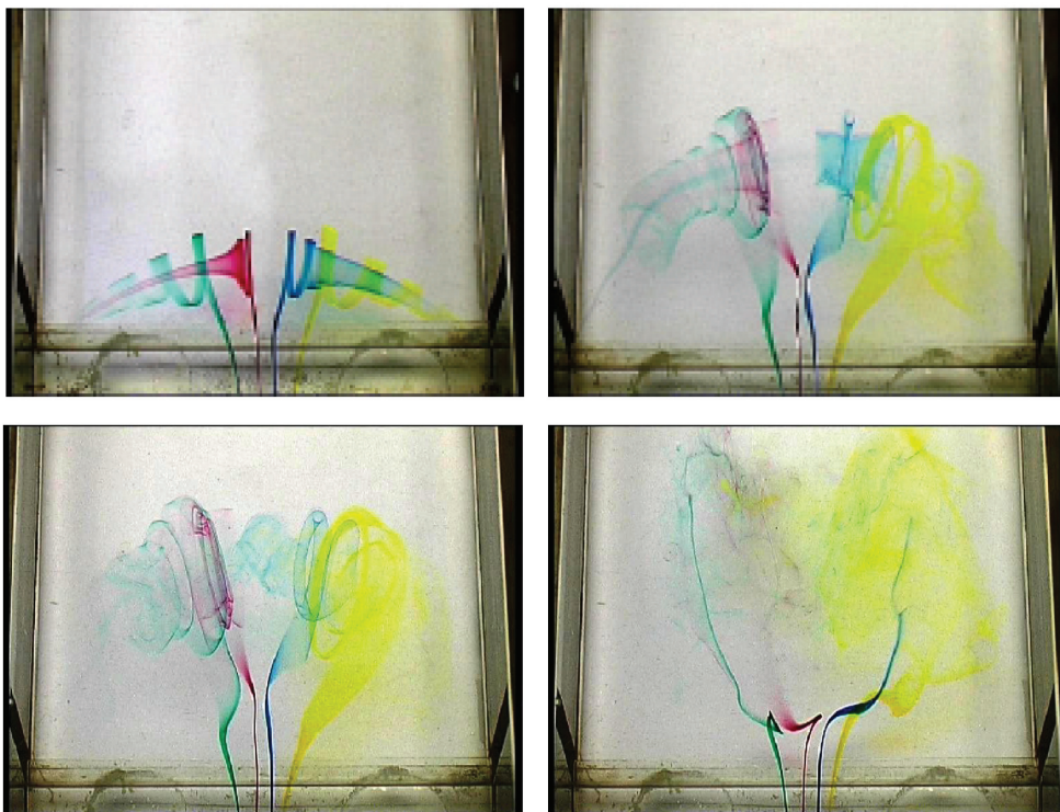
FIGURE 1. (a) Schematic of the experiment (from Cuypers et al. 2004). The vortex initiated by the step (11 mm high) is strained by the channel flow Q_1 and intensified and stretched by the axial suction Q_2 ; therefore the total flow rate through the channel is (Q_1 + 2Q_2) . The values Q_1 = 208 \text{ cm}^3 \text{ s}^{-1} and Q_2 = 125 \text{ cm}^3 \text{ s}^{-1} are chosen to produce a vortex life cycle which quasi-periodically repeats itself. (b) Time evolution of one vortex bursting. Time advances from left to right and top to bottom. Each picture is separated from the next by about 1 s. (See also movie 1 showing the experiment running.)
