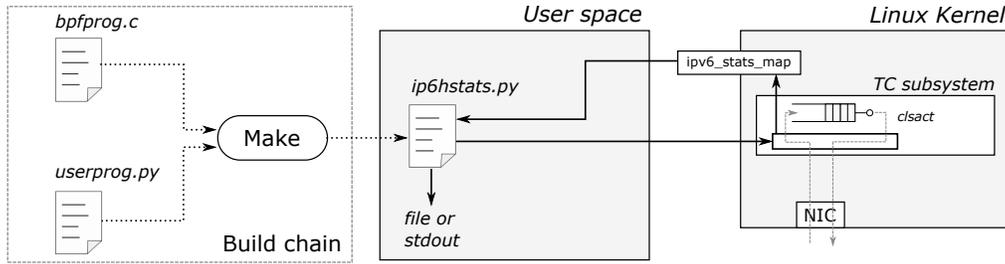
Figure 4: Architecture of the `ip6hstats.py` tool.
