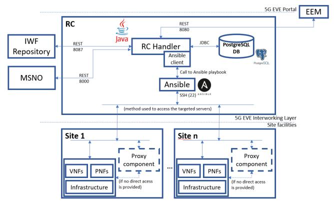
Figure 21: Runtime Configurator final architecture
