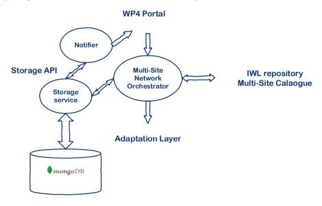
Figure 7: MSNO micro-service architecture
