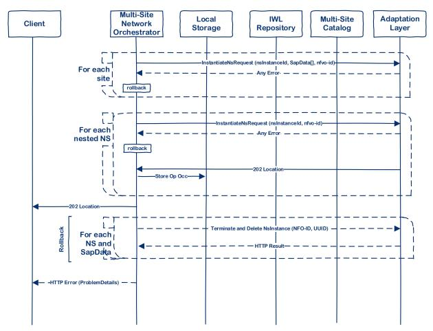
Figure 15: Workflow 2 of the Instantiation Request
