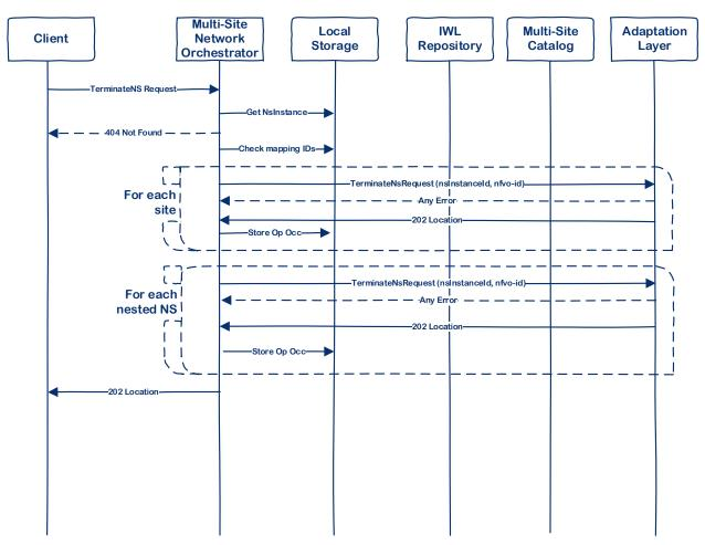
Figure 16: Termination Workflow
