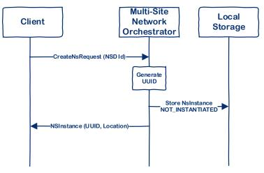
Figure 10: Create Network Service Workflow
