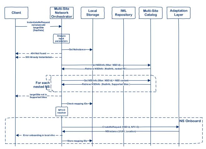
Figure 14: Workflow 1 for the Instantiate Request
