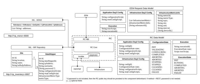
Figure 22: Runtime Configurator data model
