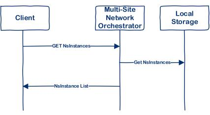
Figure 11: Workflow for the NS instances query
