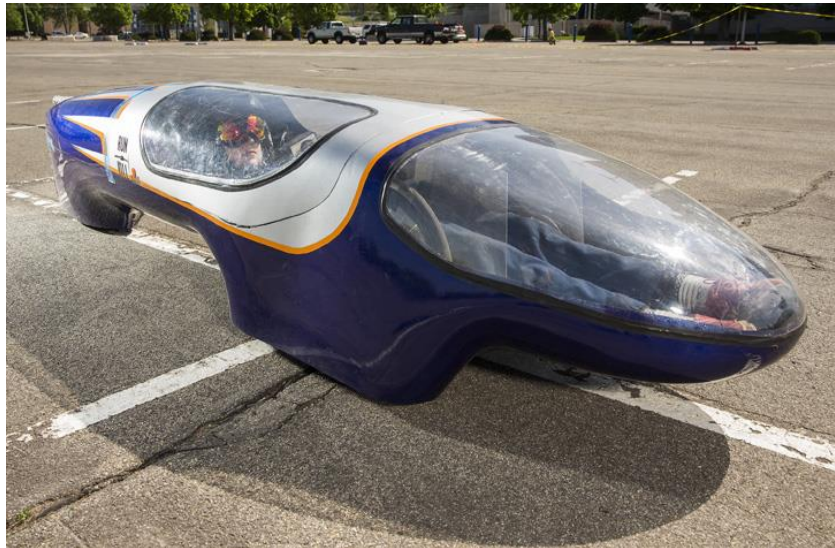
Figure 1: The 2014 BYU Supermileage Vehicle. It achieved 1300 mpg to win the 2014 SAE Supermileage competition.
