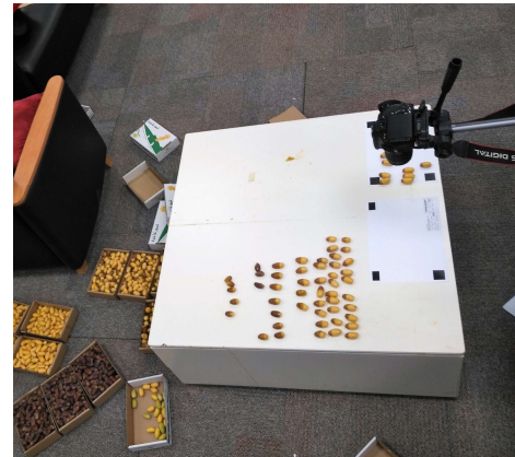
FIGURE 19. The camera position setup for the individual date imaging.
