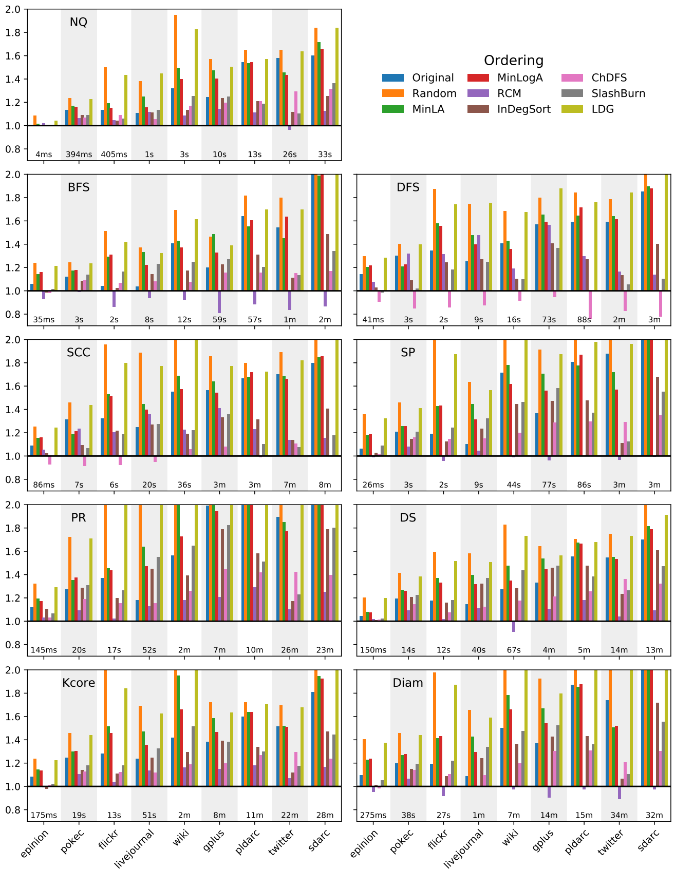
Figure 5. Speedup of Gorder. For each algorithm and each dataset, we display the absolute runtime for Gorder. Bars represent the relative time of all other orderings compared to this reference. For readability, the y-axis is cut above factor 2, but values go as high as 3.7. This figure can be compared to Figure 9 in [1]. Another visualisation is show in supplementary figure S1.
