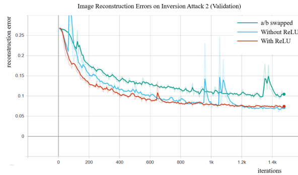
Figure 3. Training of the adversary model. Random swapping of a and b yields a significantly higher reconstruction error. The models with and without ReLU have similar reconstruction errors, but the model without ReLU needs much longer to train as it introduces better obfuscation.
