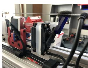
Figure 8: MechBass' servomotor-based damper
