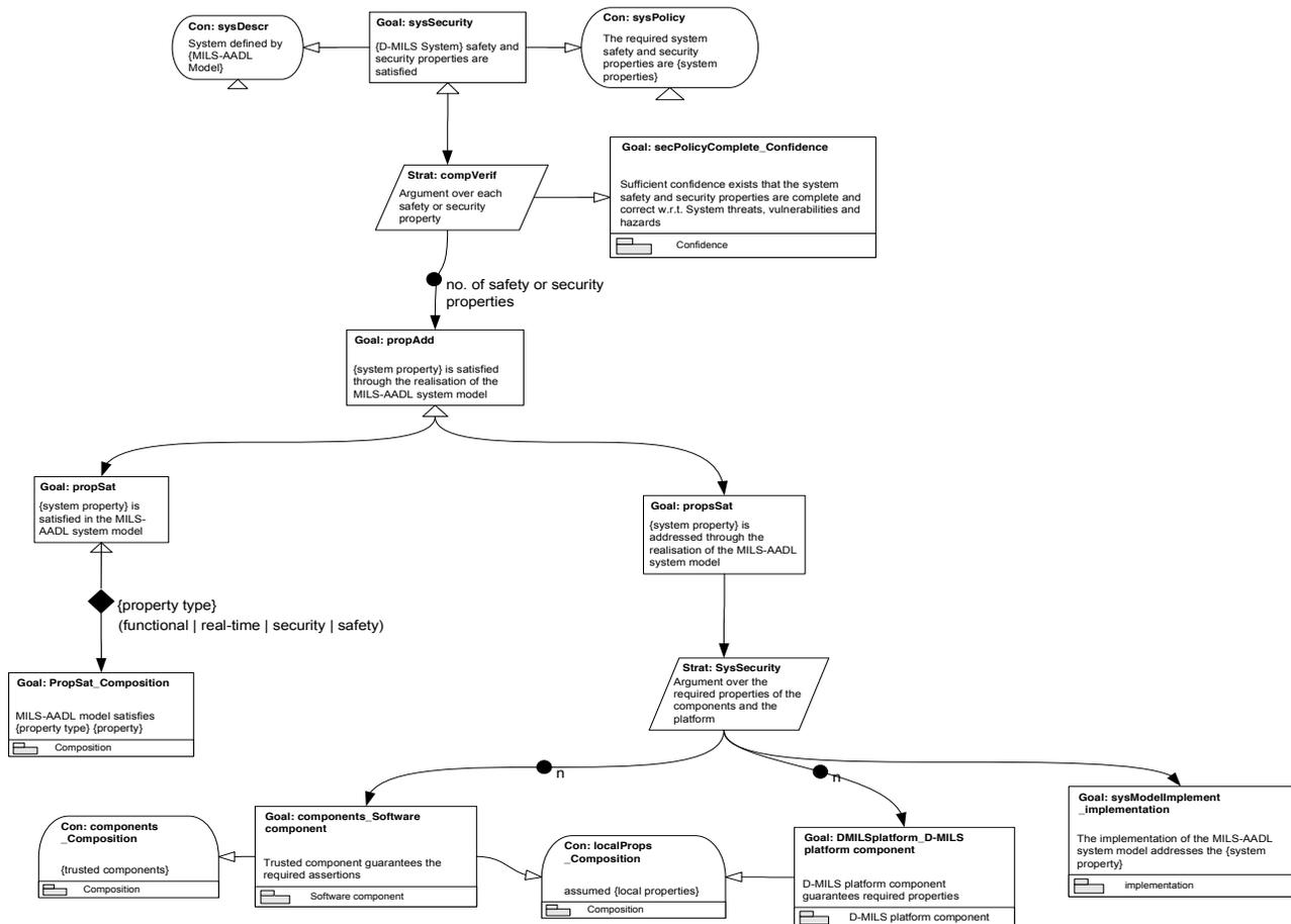
Figure 6. System properties assurance case argument pattern
