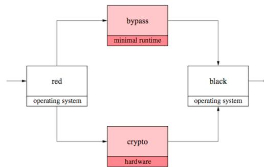
**Figure 10. Software architecture of crypto controller system**
