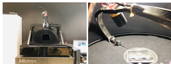
(a) Inhouse RTI dome system (b) Mechanised light source
