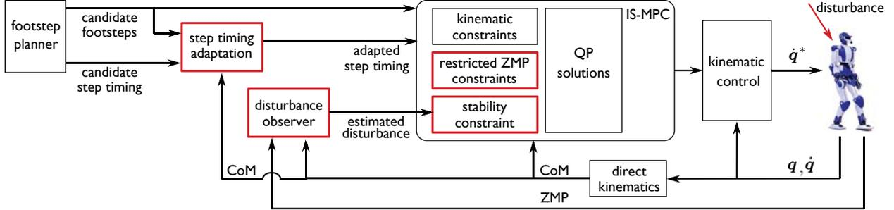
Fig. 1. A block scheme of the robust IS-MPC method for gait generation. Components added with respect to the original scheme are shown in red.
