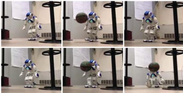
Fig. 3. NAO is hit by a ball while walking: robust IS-MPC (top), nominal IS-MPC (bottom). Thanks to the step adaptation module, IS-MPC is able to preserve feasibility by reducing the step duration, while nominal IS-MPC fails causing the robot to fall.
