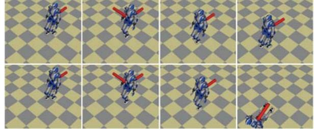
Fig. 4. HRP-4 walking under multiple pushes: robust IS-MPC (top), nominal IS-MPC (bottom). The robot is walking under a constant disturbance in the  $x$  direction and an impulsive disturbance in the  $y$  direction. Robust IS-MPC is able to successfully withstand the disturbances, while the nominal scheme fails.
