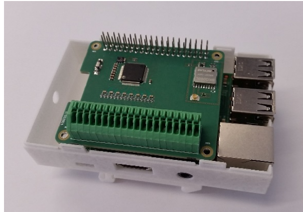
Figure 35: Embedded solution for PMU applications.
