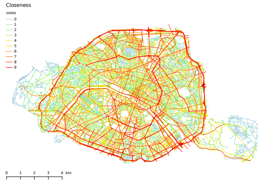
Fig. 1. Closeness indicator applied to the network of reconstructed ways of the city of Paris. This indicator reveals in parts the history of this network: The oldest ways and main piercings have a high score (in red), they are the most accessible in a small number of turn for the whole. network.
