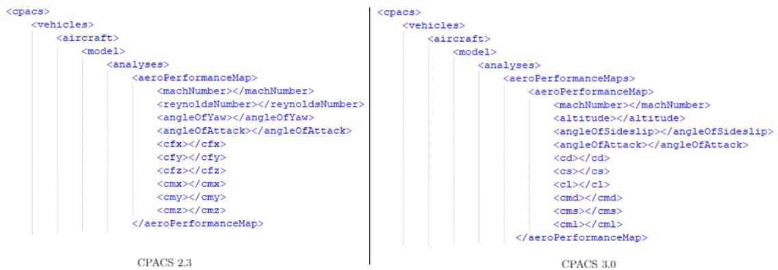
**Figure 4.20:** Comparison between CPACS 2 and 3 schema for the section which describes aircraft aerodynamic performance. It is possible to notice a slight difference between the two versions [40].
