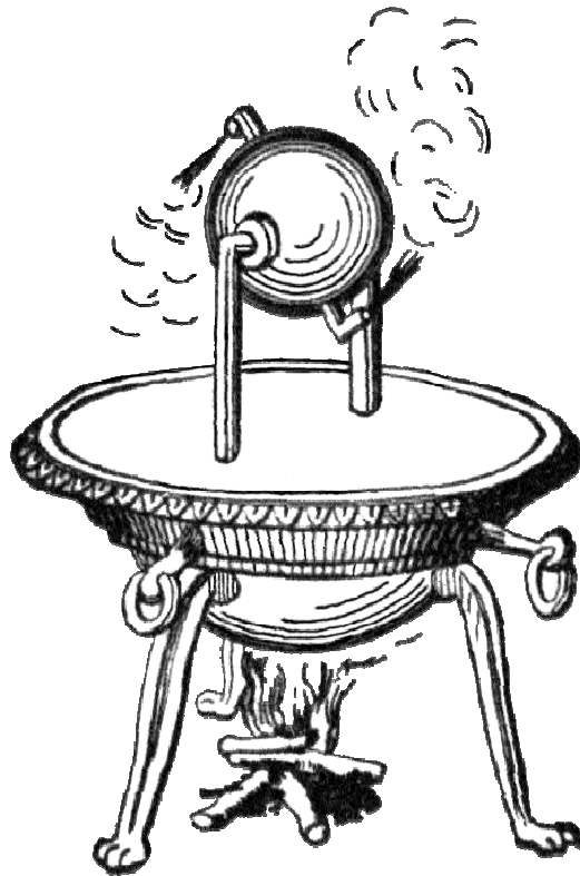
Figure (1) Sketch of the first known steam machine designed by Hero during the first century BC.
