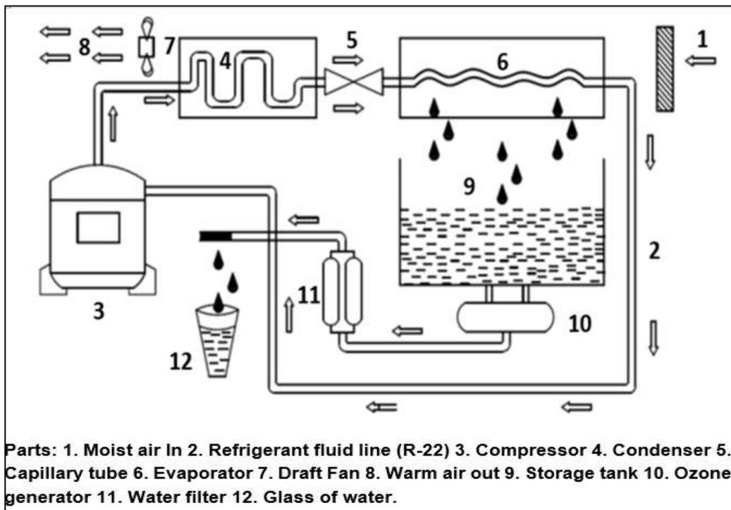
*Fig.2(a):-Schematic view of the experimental set up*
