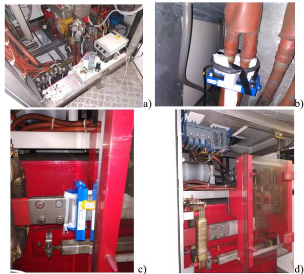
Fig. 2. Voltage transducers and measurement supply system a) current transducers for rheostat monitoring b), transducer for current measurement at the pantograph c), Compact Rio arrangement d)
