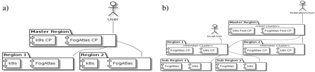
Fig. 1. a) Scenario 1: FogAtlas handles a single Kubernetes cluster covering the entire infrastructure; b) Scenario 2: The infrastructure is divided in different independent and federated Kubernetes clusters.
