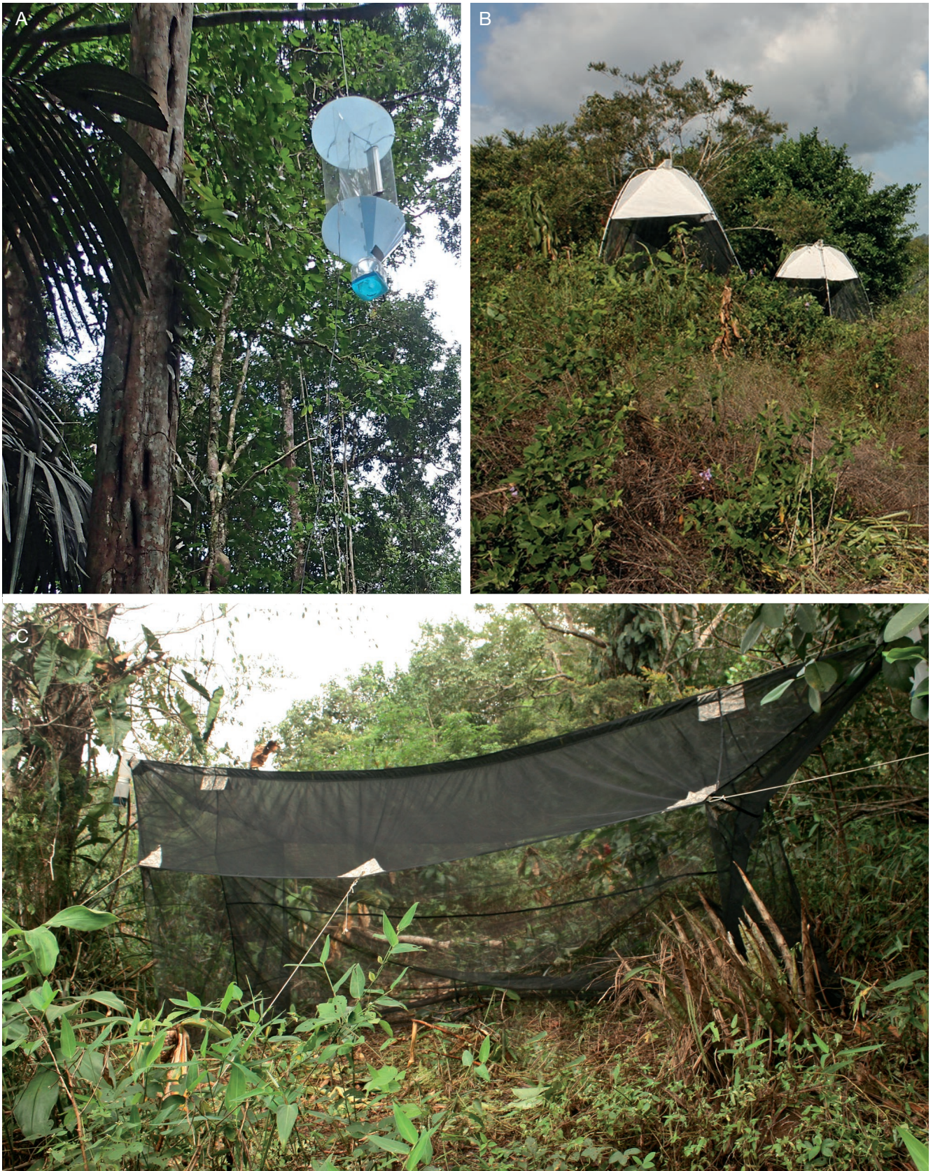
FIG. 5. — Collecting techniques that yielded Agromyzidae Fallén, 1823 samples in Mitaraka: A , PVB light trap; B , SLAM traps; C , 6 m long Malaise trap (Photos: A, Julien Tourout; B, C, Stéphane Brulé).
