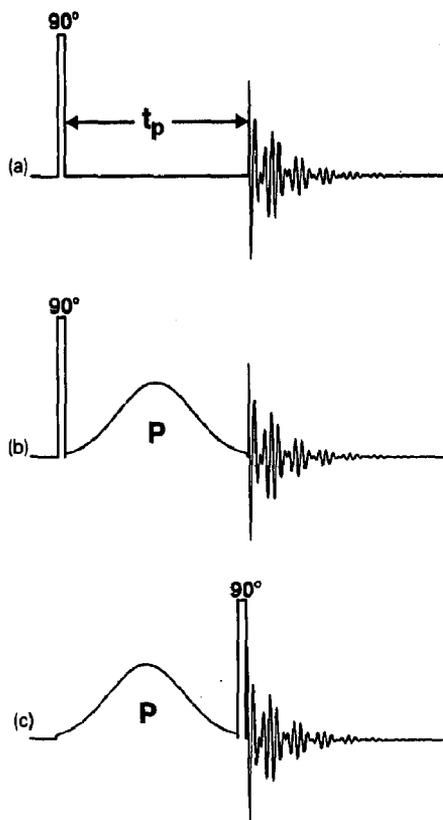
Fig. 1. Experimental schemes suitable to demonstrate transient Bloch-Siegert effects. (a) Hard  $90^\circ$  pulse followed by acquisition after a delay  $t_p$ . (b) Hard  $90^\circ$  pulse followed by application of a time-dependent irradiation P of duration  $t_p$  before acquisition. (c) Same as (b) but with permutation of the hard and soft pulses. The pulse P is shown as a truncated Gaussian, but it could be defined by an arbitrary envelope function.
