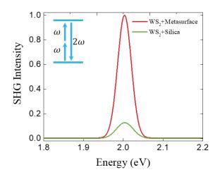
**Fig. 4** | **SHG enhancement in synthetic metasurface**. The SHG signal from WS<sub>2</sub> on top of the Au metasurface (red line) and the silica (green line). The fundamental energy of excitation signal is 1.002eV.
