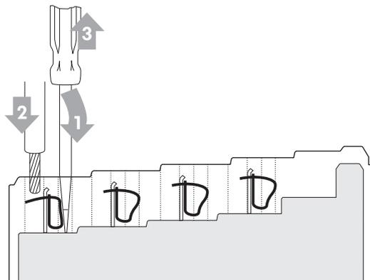
Figure 35: Connecting a conductor to a CAGE CLAMP®
