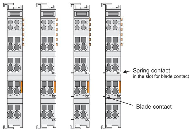
Figure 34: Example for the arrangement of power contacts
