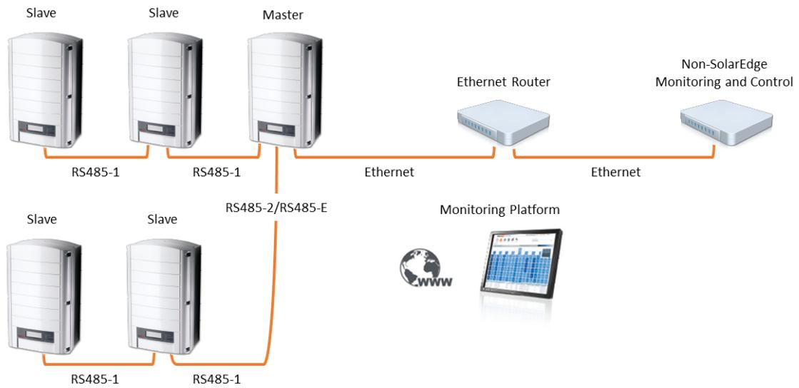
**Connection to the SolarEdge monitoring platform and to a non-SolarEdge monitoring device using a Commercial Gateway**
