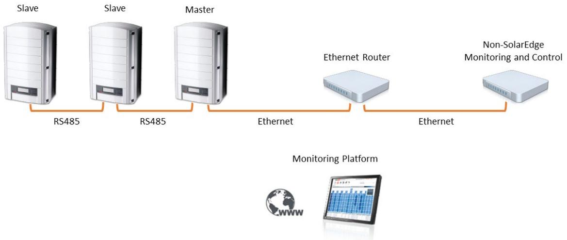
Connect a second chain of the inverters to the Master inverter using RS485-2/RS485-E.
