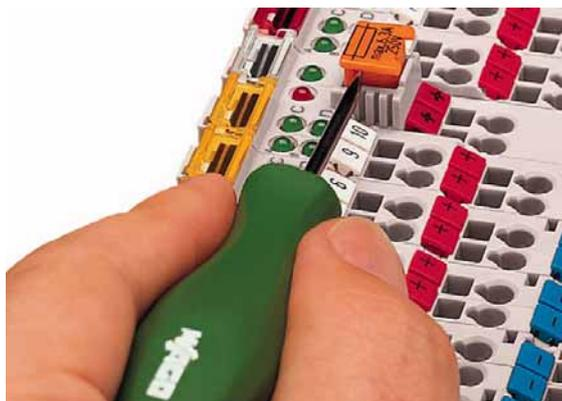
Figure 8: Removing the fuse carrier
