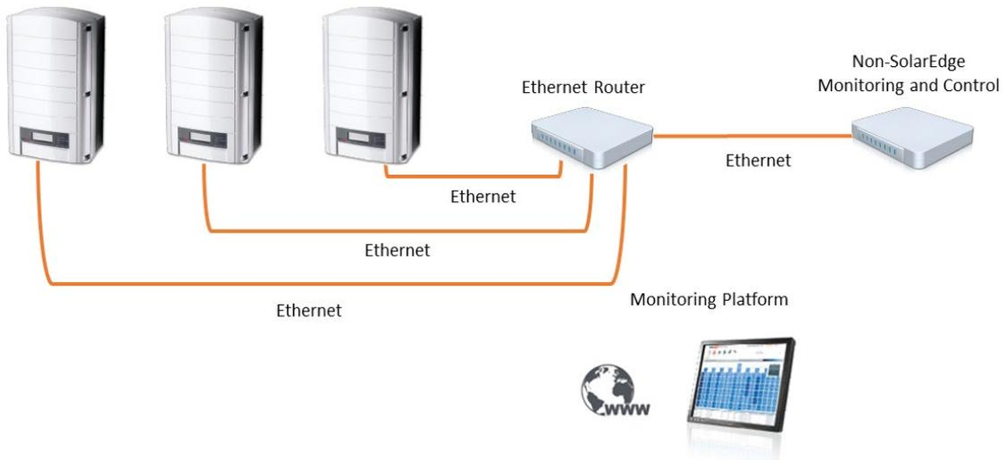
**Option 2** – Connect the Master only to the Ethernet router via Ethernet cables.
