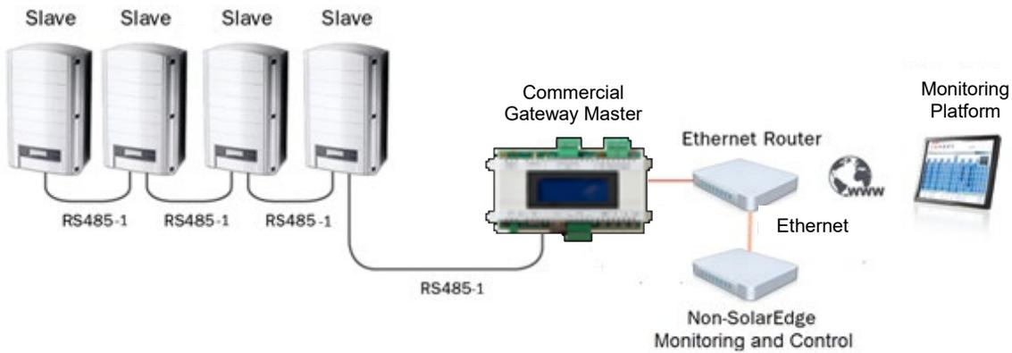
If required, use the RS485-E bus for connecting a second chain of inverters.
