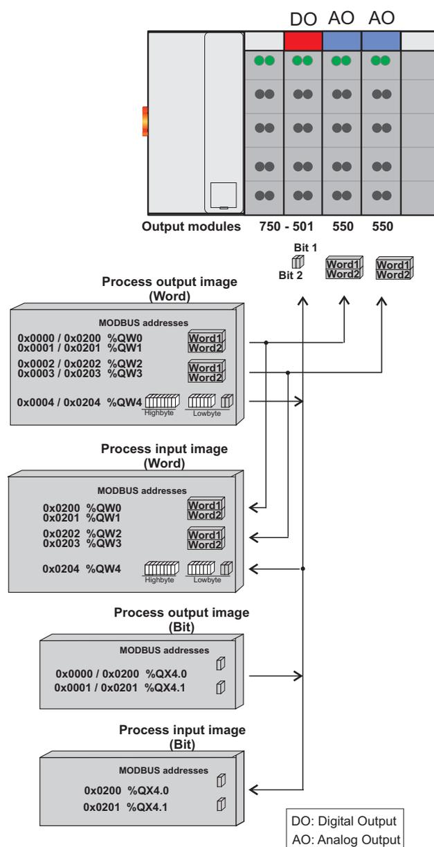
Figure 38: Example of process image for output data
