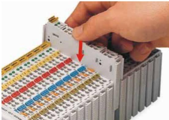
Figure 31: Snap the I/O module into place
