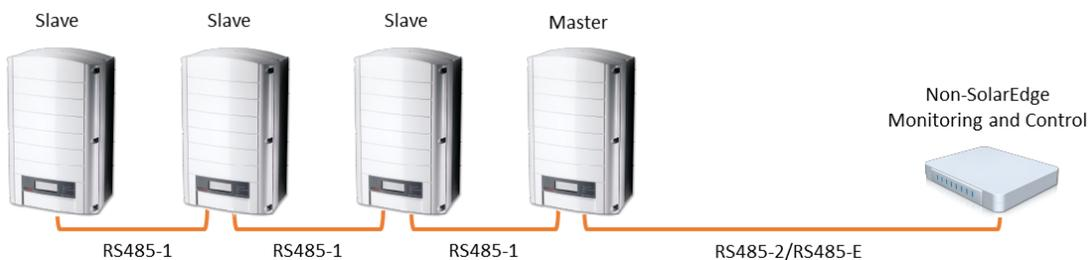
**Connection to a non-SolarEdge monitoring device (with connection to the monitoring platform)**
