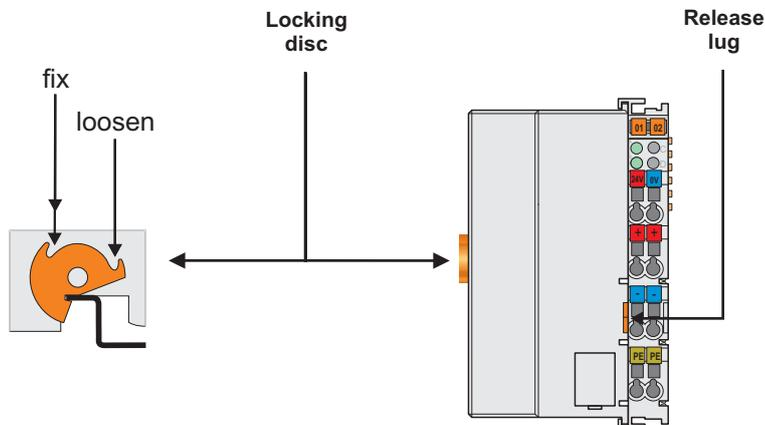
Figure 29: Unlocking lug of extended ECO coupler
