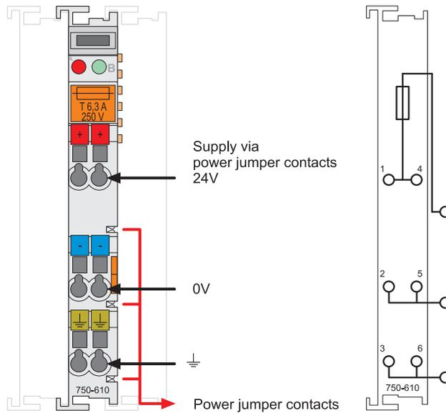
Figure 7: Supply module with fuse carrier (Example 750-610)
