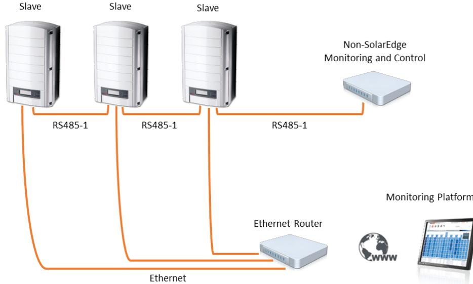
**Option 2** – Connect the Ethernet router to one inverter only.
