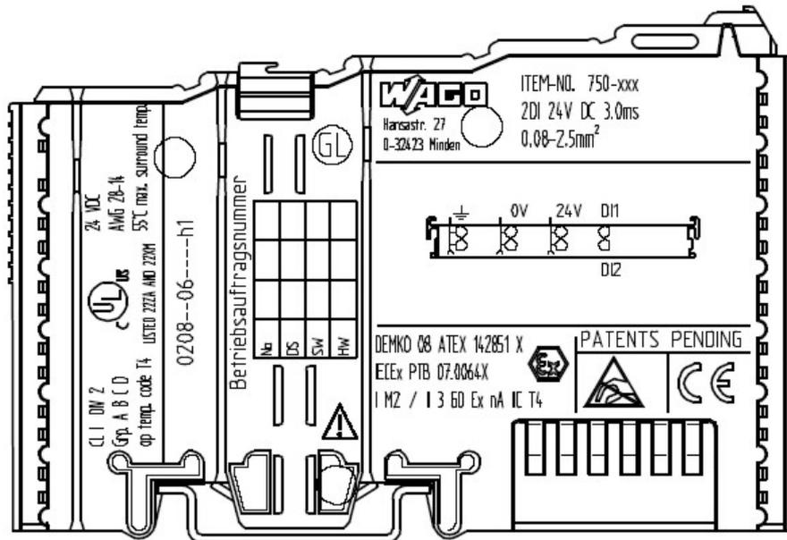
Figure 78: Side marking example for ATEX and IEC Ex approved I/O modules according to CENELEC and IEC
