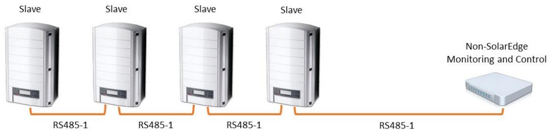
**Option 2** – Use RS485-1 to connect slaves to the master; use either RS485-2 or RS485-E to connect the master to a non-SolarEdge monitoring device. Every inverter in the RS485 bus should be configured to a different device ID (MODBUS ID).
