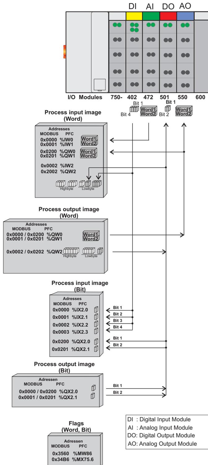
Figure 44: Example of addressing for a fieldbus node
