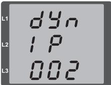
Fig.: Parameter setting for dynamic allocation (DHCP) of a TCP/IP address
