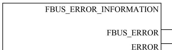
Figure 75: Function block for determining loss of fieldbus, independently of protocol
