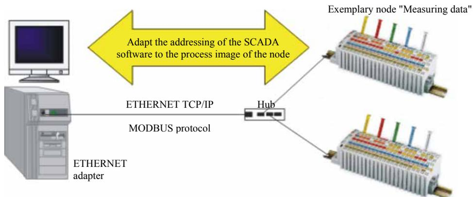
Figure 77: Example SCADA software with MODBUS driver
