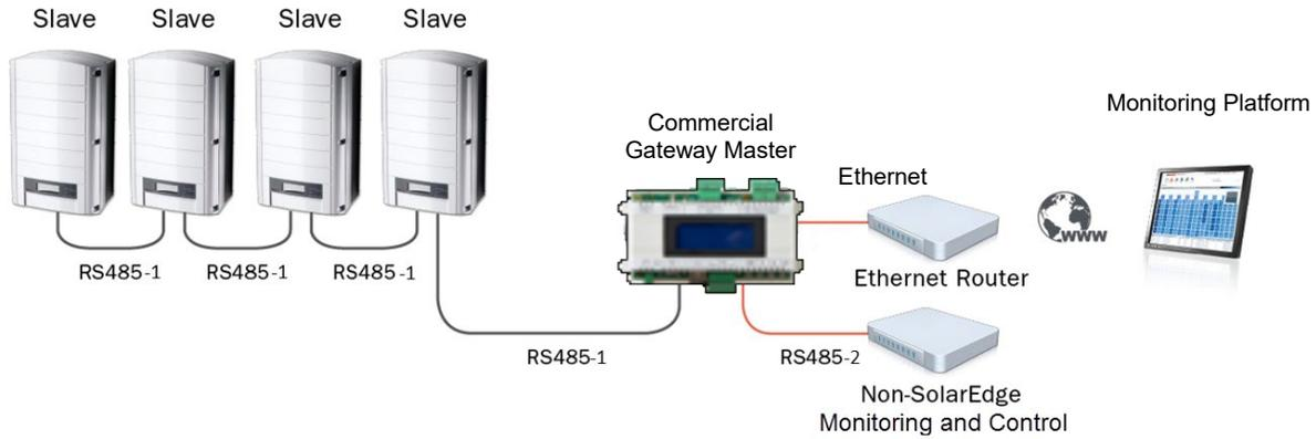
If required, use the RS485-E bus for connecting a second chain of inverters.
