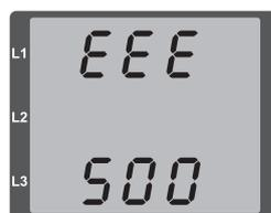
Fig.: Warning message with number 500 (mains frequency)
