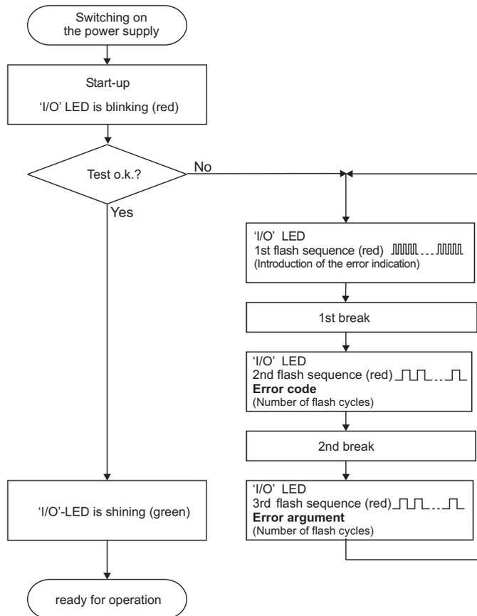
Figure 73: Node status - I/O LED signaling
