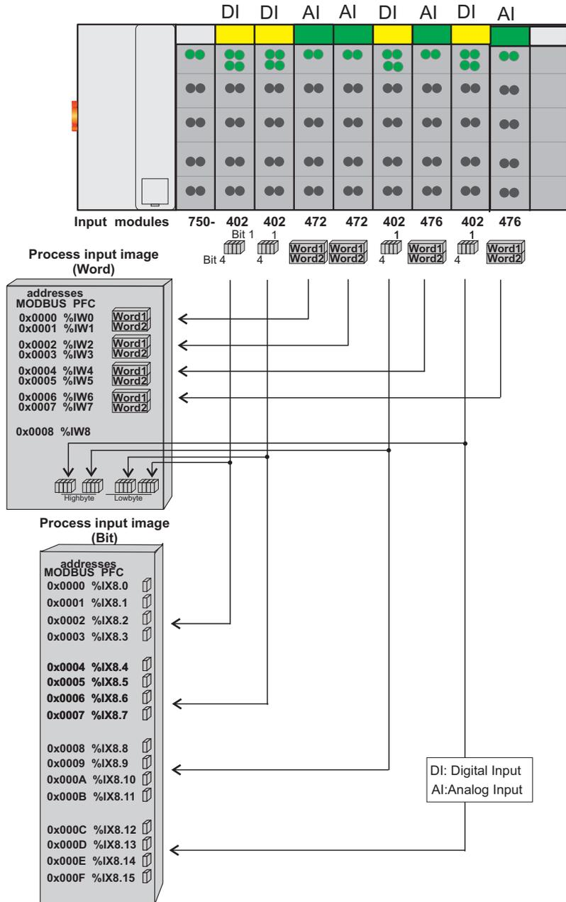
Figure 37: Example of process image for input data
