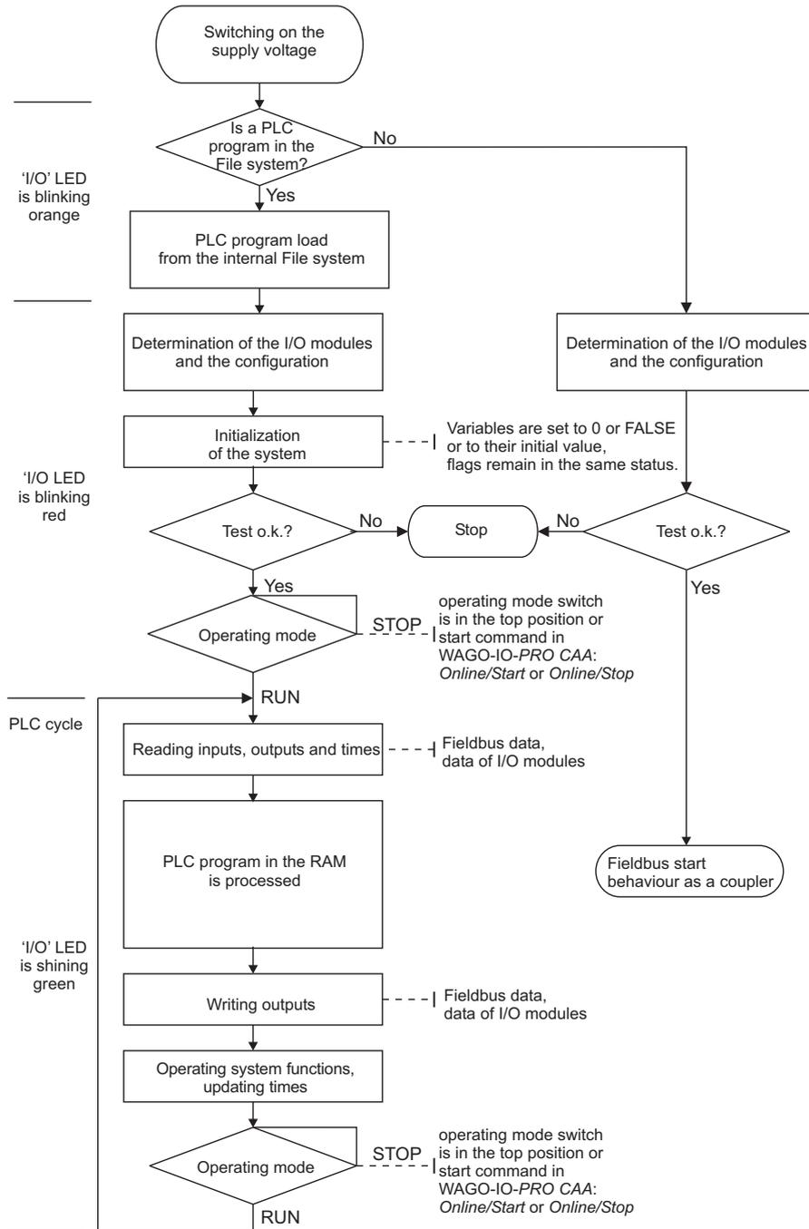
Figure 36: Run-up of the Controller
