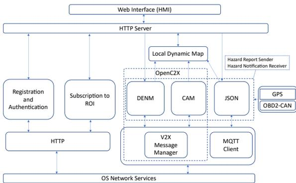
Figure 2: Software architecture of the OBU.
