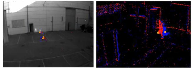
Fig. 4: Frame-based image and event stream obtained in surveillance experiments performed in the day (left) and in the night in total darkness (right).
