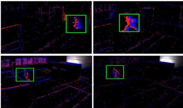
Fig. 7: Detection and tracking results in dark (top) and dynamic (bottom) lighting conditions experiments.
