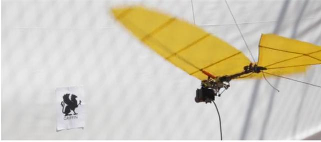
Fig. 3: Set-up of the motion-blur experiment with a DAVIS 346 sensor onboard a flapping-wing ornithopter.
