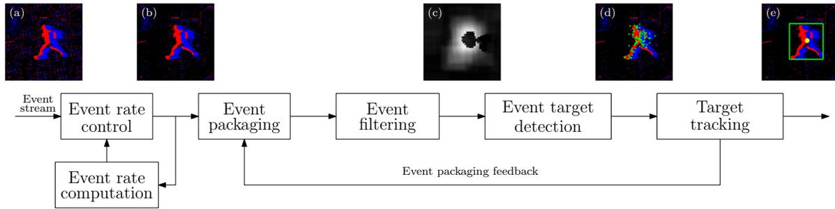
Fig. 2: Event-based target detection and tracking scheme: a) event stream representation, b) event stream representation after random discard procedure, c) APM obtained for event filtering, d) corner tracking, e) event clustering and, f) target tracking.
