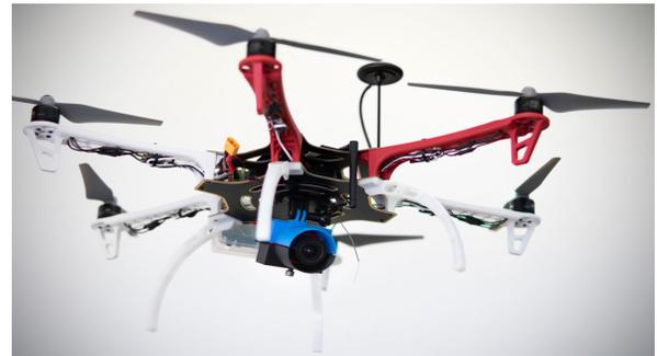
Fig. 5: Robot used in the shown experiments: a DJI Flamewheel F550 platform with a DAVIS 346 and an INTEL NUC.
