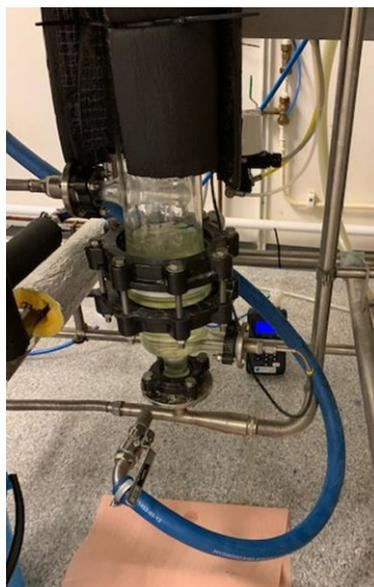
**Figure 4** CHE626 automated absorption and stripping pilot plant operating at batch mode (recirculation).
