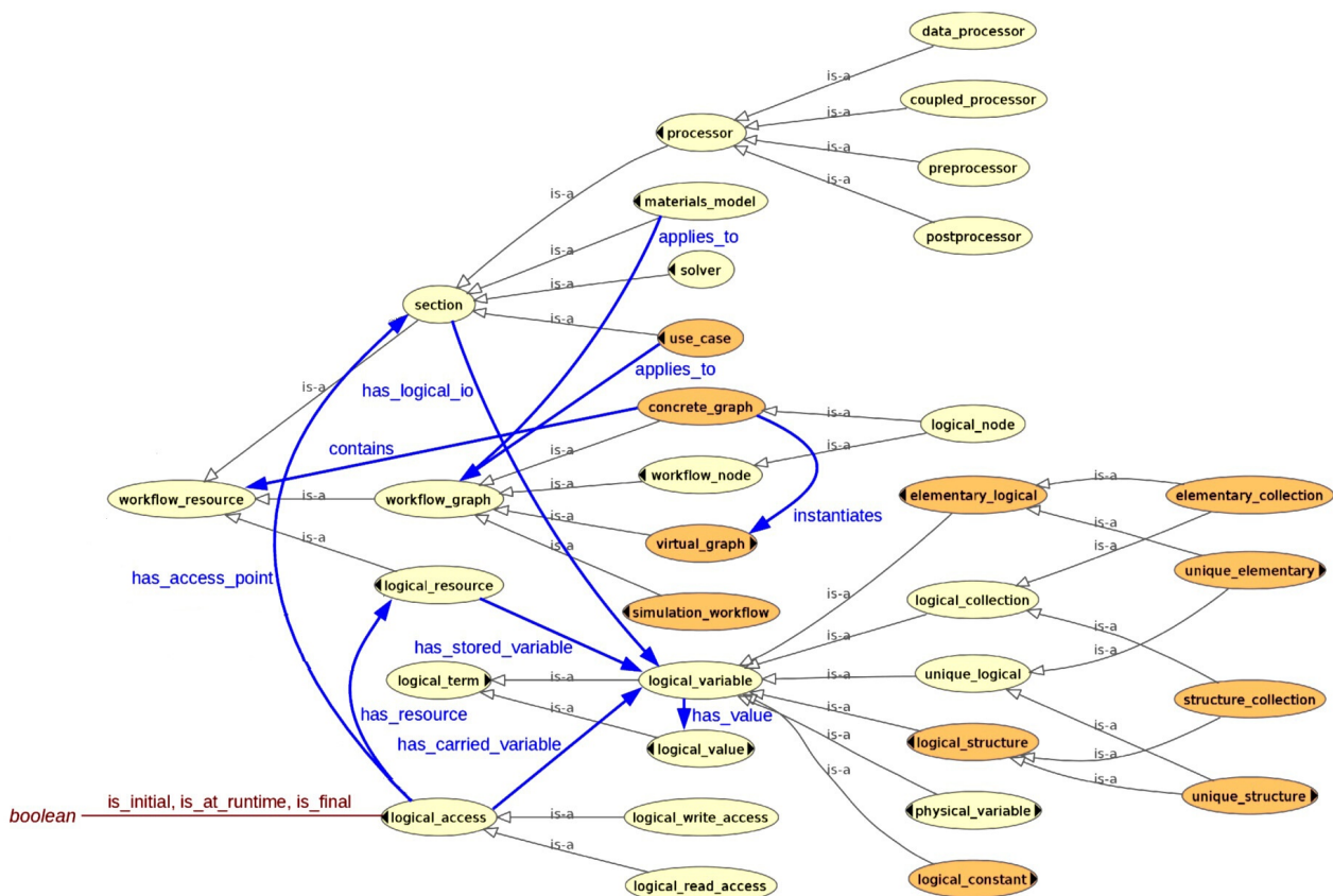
Figure 3.8. Workflow resource branch of OSMO [Hor20b]: Selected concepts (ellipses), relations (blue arrows), and datatype properties (solid line); the diagram was generated using the OWLViz protégé plugin; grey arrows labelled "is-a" denote subsumption ( \sqsubseteq ), i.e., \text{rdfs:subClassOf} .
