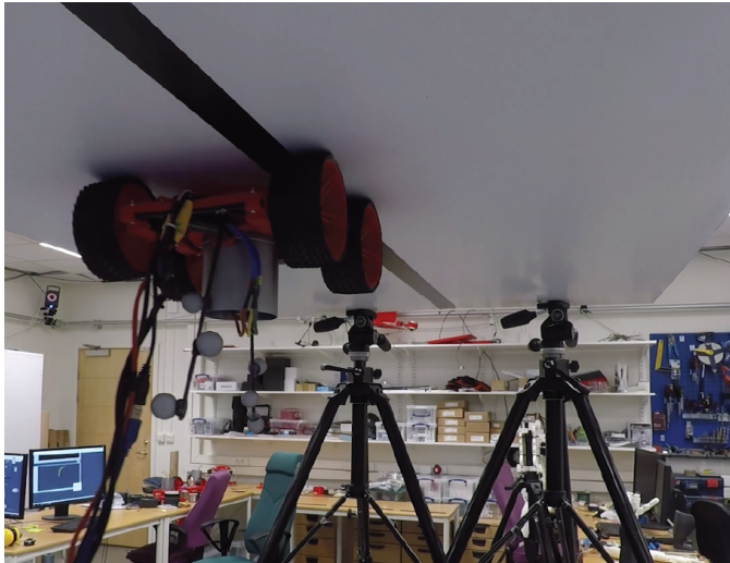
Fig. 6. VRP under experimental evaluation on an inverted flat surface
