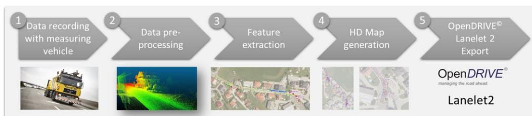
**Figure 4 – Uniform process chain for generating the high definition digital map**
