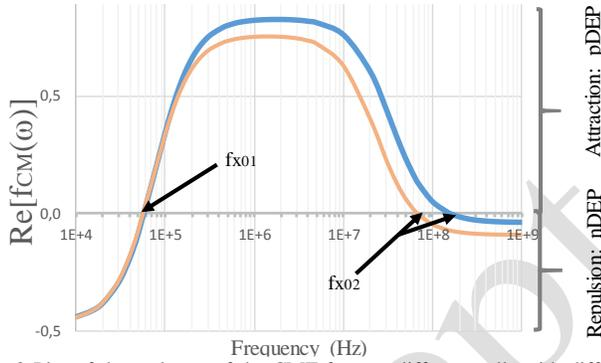
Fig. 2 Plot of the real part of the CMF for two different cells with different cytoplasm dielectric properties.
