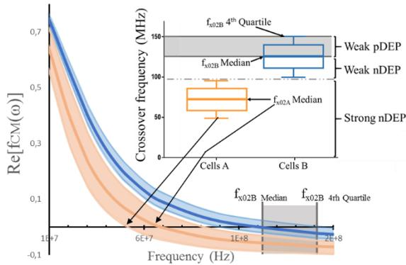
Fig. 4 Plot of CMF and dispersion of  $f_{x02}$  for two different cell types. The grey frequency range corresponds to proper DEP frequencies.
