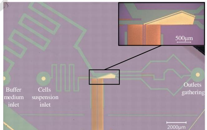
Fig.1 Photograph of the proposed cytometer prototype.
