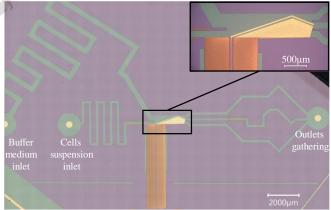
Fig.1 Photograph of the proposed cytometer prototype.
