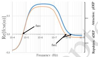
Fig. 2 Plot of the real part of the CMF for two different cells with different cytoplasm dielectric properties.
