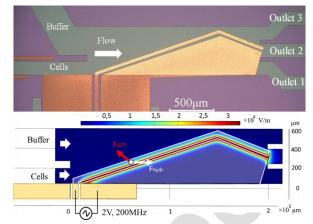
Fig. 5 Top view of the cytometer main sorting area and associated E field distribution plot. The electrodes have been drawn clearer with white edge.
