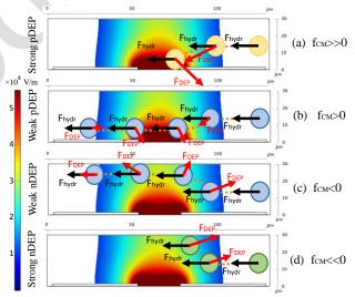
Fig.3 Electric field influence on the flowing cell trajectory related to its CMF value. COMSOL Multiphysics simulation for 2V applied signal.
